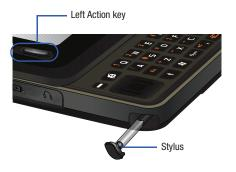
Use your stylus to calibrate the touch accuracy of the screen by both accurately and firmly touching the center of each onscreen crosshair. Repeat this process for every crosshair that appears until this step has successfully completed.
